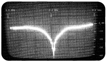
Photo 8. Circular-polarized patch frequency response.
