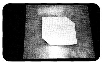
Photo 7. A 2.4-GHz circular-polarized patch.
