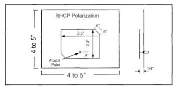
Figure 3. Circular-polarized patch dimensions.
