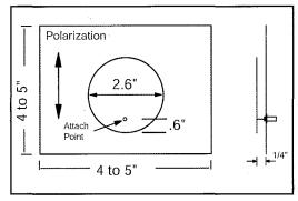
Figure 1. Circular patch dimensions.
